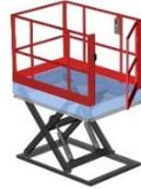
A safety door is usually combined with a rail and secures the side via which loading or unloading takes place when the platform is in a raised or lowered position. Safety doors are often fitted when the lift table is used as a working platform. The door is locked by means of a safety lock, which only opens when the lift table is in a secure position.
