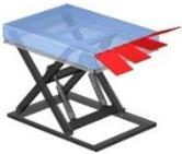
Segmented tailboards are an effective way of bridging the gap between the vehicle and the lift table. The standard segment split is usually approx, 400x400 mm. The max. load capacity of a single segment is 750 kg. For lift heights of < 1600 mm, the side facing towards the vehicle can be left open without the need for any securing rails or safety doors.
