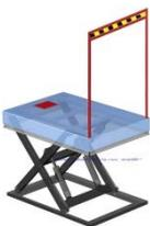
A portal bridge is used as a safety rail for the side of the lift table next to the ramp and prevents the ramp area from falling when the lift table has been completely lowered. Depending on the type of ramp used, the clear passage height is the effective lift height + 1100 mm.
